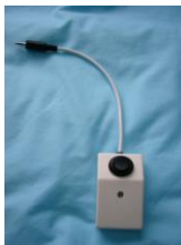
Customer service/panic switch
